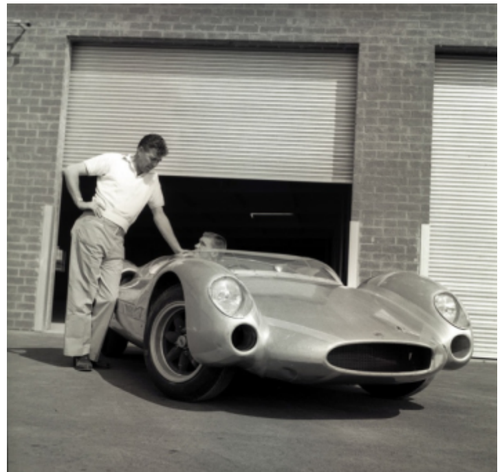
Carroll Shelby (L) and Dave MacDonald (seated) with the short-lived Cooper Monaco (King Cobra) project in 1963. Oh, it was fast alright – that wasn't the problem. The King Cobra was powered by a “full race” 289 cu/in Ford engine & Huffaker 4-spd transaxles (later swapped out for a Colotti transaxle) that sat atop the beefed-up Cooper chassis & suspension. The car handled horribly – there wasn't enough rubber or weight to handle the hulking horsepower.
