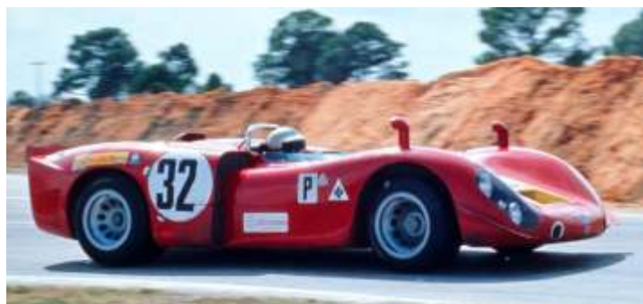
The beautifully painted Lola T70 Mk.3B of Ulf Norinder and Jo Bonnier broke a radius arm mounting and had to retire. Sebring was notoriously rough in those days.
