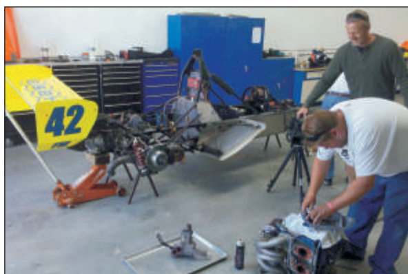
Engine out. Dan replacing seal & gasket
